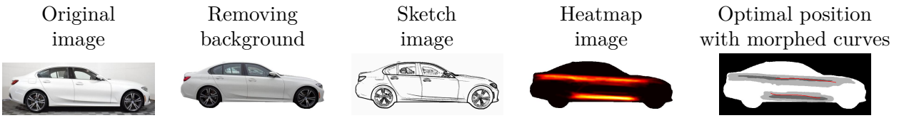
Figure 12: Key Steps of Generating a Bio-Inspired Facelift Design for a Given Morphing Degree
